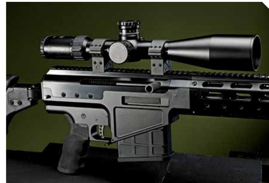
The massive receiver is machined out of a solid block of 9310 steel. The magazine well is cut at an angle to allow easy magazine insertion and extraction from the prone position.
