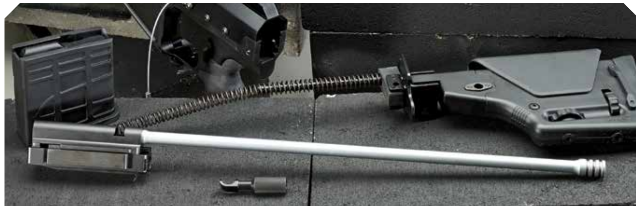
The heart of the Alexander Arms piston system is its beefy, 16½-inch operating rod attached to a solid block/bolt of stainless steel.
